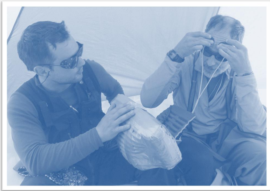
Nonin Equanox Model 8000CA cerebral oximeter in use. Note padded cover (made from sleeping pad material and duct tape) for insulation and impact resistance
